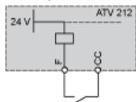
“PLC” position with PLC transistor outputs
